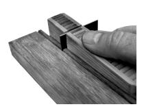
those made by a card scraper. When it no longer produces shavings, the cutter should be re-sharpened.
