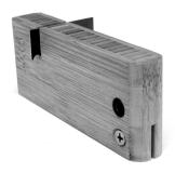
The Scratch Stock is an old tool dating back centuries to a time when furniture was made one piece at a time in the workshops of master craftsmen. It was used to shape edge profiles, cut grooves for inlaid stringing, and many other such detailed tasks. Although the Scratch Stock
