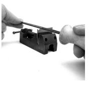
that are straight can be cut with rectangular, square, or triangular files. Radius sections require a round file. Common rat-tail round files are tapered and do *not* work well. Instead, use chainsaw files, which are parallel-sided, have fine teeth, and are available in a wide variety of sizes. Dremel-type hand grinders can also come in handy here.
