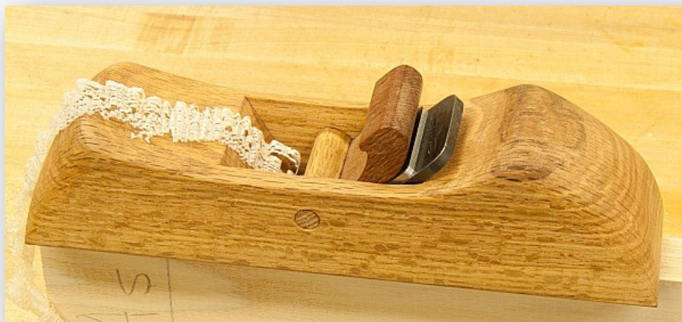
The body for Mark Ketelsen's 10" x 2-3/8" smoother is from a piece of swamp white-oak from his firewood pile. The wedge is leopard wood and the sole lignum vitae .
