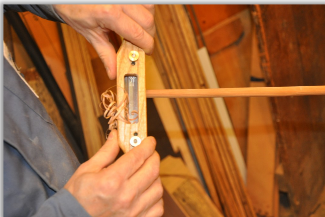
Vincent Lavarenne gets sweet, curly shavings as he shaves a spindle with his new spokeshave set with a Hock Tools spokeshave blade .
