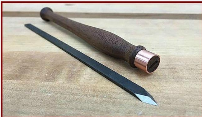
**Scott's Marking Knife disassembled. Note the copper ferrule and the perfectly sized mortise.**
