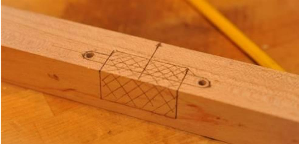
**Figure 1: Center line, 3/8" line, blade outline, throat definition.**
