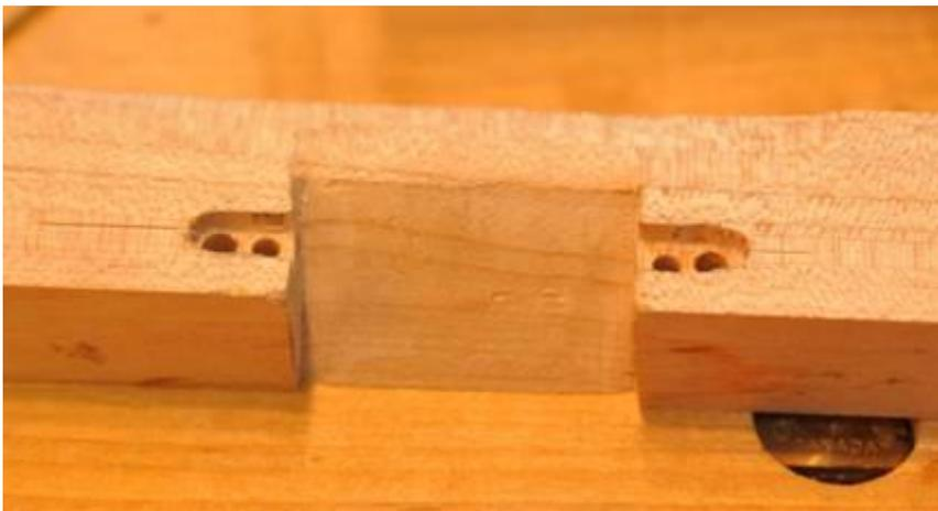
Figure 3 Showing set screw holes
