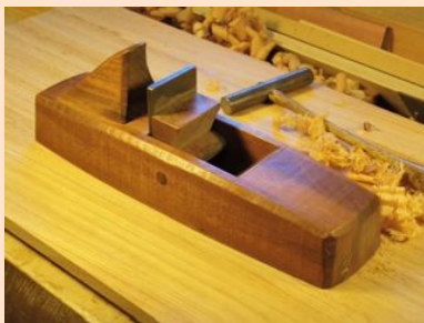
“When wood is a challenge to plane, this brawny fellow is the efficient solution. With a Hock iron at 90 degrees, sharpened at a steep 45, this scraper plane will flatten the most difficult of woods. Large, easy to use and keeps an edge.”
