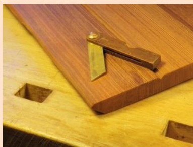
"One of several bevel gauges hanging on my wall, but this one is most used. Small, sweet and easy to make."
