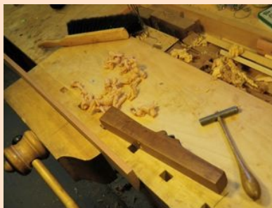
"A jointer plane for narrow edge joints, including band saw veneer joints. Possibly the best plane I have ever made. The hammer I use to adjust my planes. Made from hickory and soft steel. Incredibly comfortable in my hand. The thin shaft is springy, making it perfect for copper riveting in boat building."
