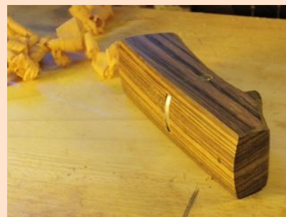
“A compass cooper plane in zebra wood. I made this one a few years back for hollow carving oar spoons. I had bought a Veritas hollowing plane, but even though it's a decent tool, it was also wicked uncomfortable in the long run. This little plane is the sweetest thing to use and works just right.”
